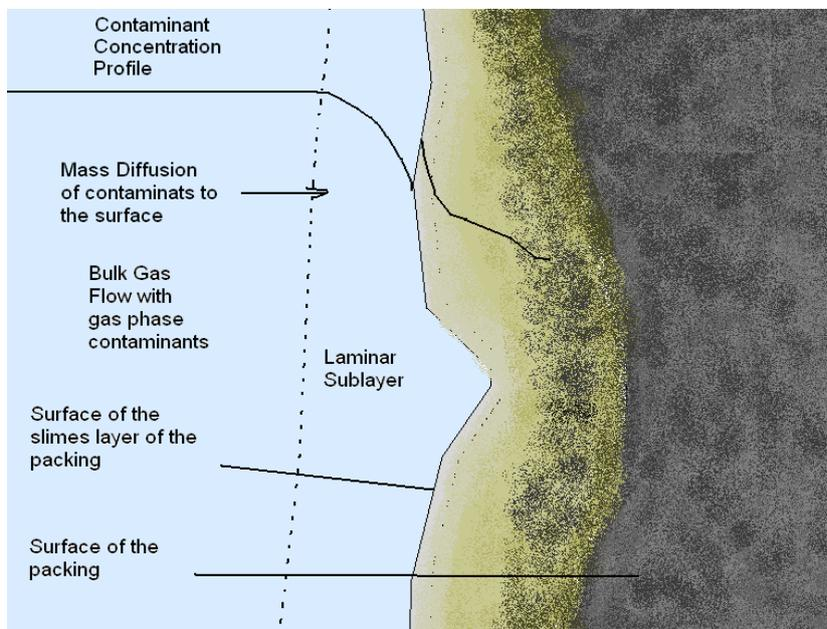
The likely mechanism is where moisture is only sparingly used and that there is direct contact between the gas phase and the surface membrane of the bacteria allowing adequate performance of the system.
